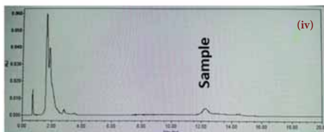
Analytic method standardization for Bisphenol A: i) Linearity of BPA in Methanol by using HPLC-PDA system; ii-iv) BPA chromatograms in HPLC
