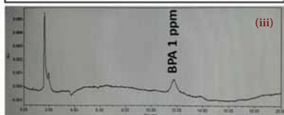
Analytic method standardization for Bisphenol A: i) Linearity of BPA in Methanol by using HPLC-PDA system; ii-iv) BPA chromatograms in HPLC
